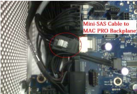
Figure 1 – iPass cable disconnected from motherboard
